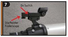
Once you have aligned your finderscope, make sure to turn off the LED light to conserve the battery. Now you are ready to align the telescope. This will have to be done at night.
